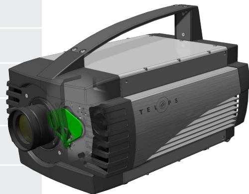
The automated 3-position filter mechanism.
