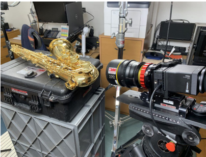
Tokina 100mm Macro lens exposed at F22 for maximum DoF. 6" to front element and 14" to image plane. Shallowest DoF of 3 examples.
