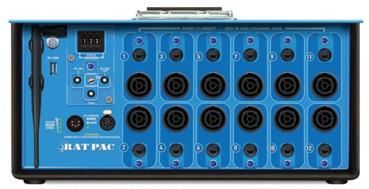
The 12x200W offers a smooth dimming curve from 100% down to 1%. USB out for convenient device charging- all in one small but powerful dimmer. ETL and CSA listed. Transmit or receive with the flip of a switch using CRMX wireless DMX technology.
