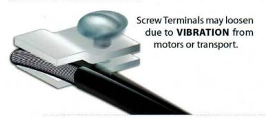
After screw termination is made, the fine copper strands tend to shift, allowing the screw to loosen. This phenomenon is called CREEP. It leads to heat rise, more loosening, and often device failure.
